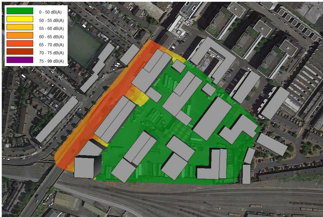
Figure 9 Predicted Noise Contour Across the Developed Site – Night
