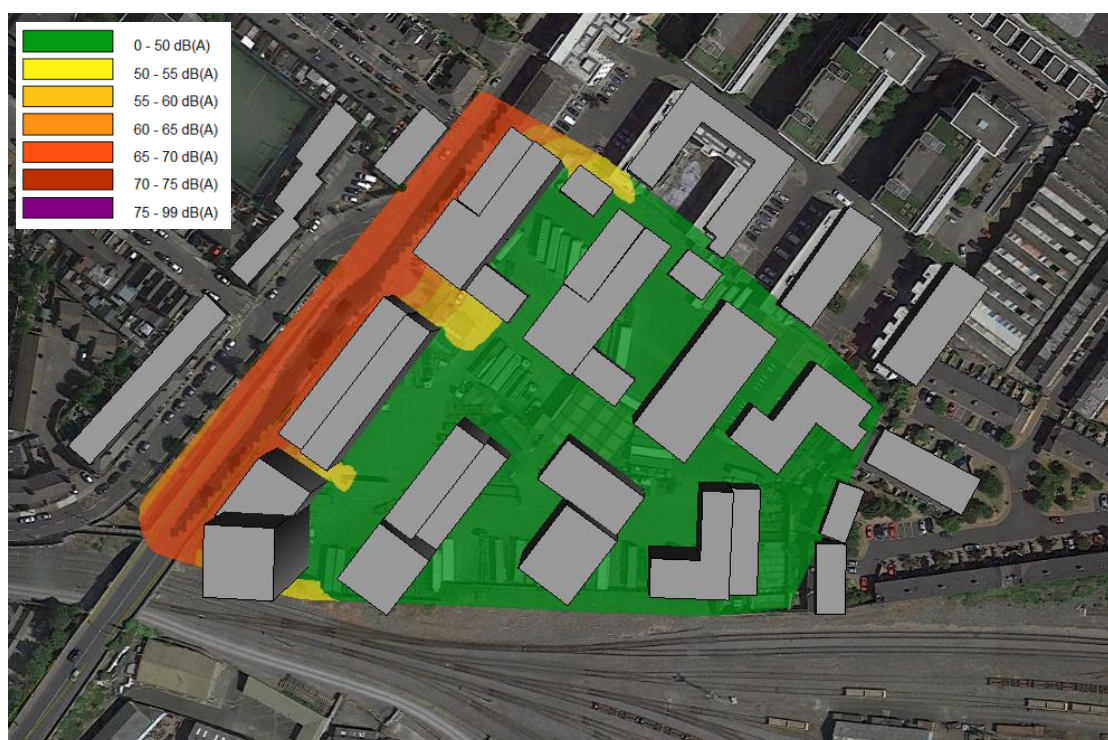
Figure 8 Predicted Noise Contour Across the Developed Site – Daytime
